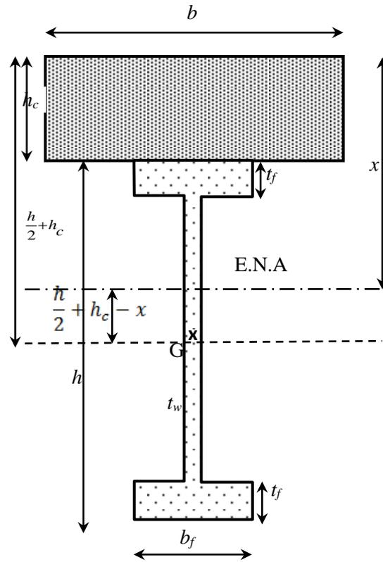
**Figure 2:** Elastic design of cross section of composite beam (serviceability limit states (SLS))
