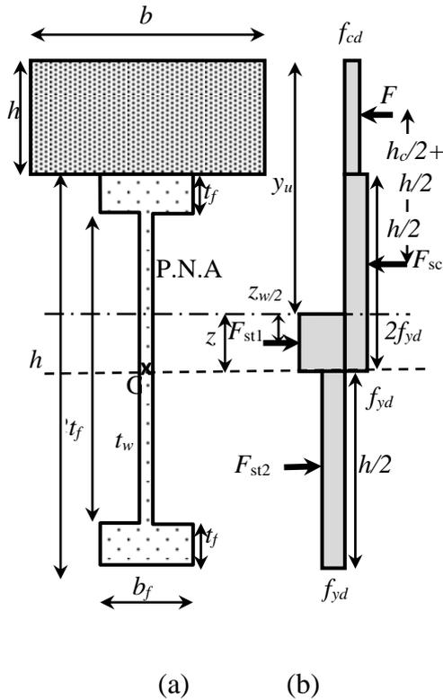
**Figure 1:** (a) Notations for composite beams;
