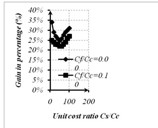
**Figure3:** Variation of relative gain in percentage versus two unit cost  $C_f/C_c$  ratios, for different values of  $C_s / C_c$ .
