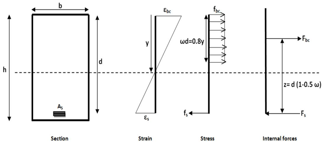
Figure 2. Typical rectangular section, strain, stress and internal force distributions under ultimate design load.
