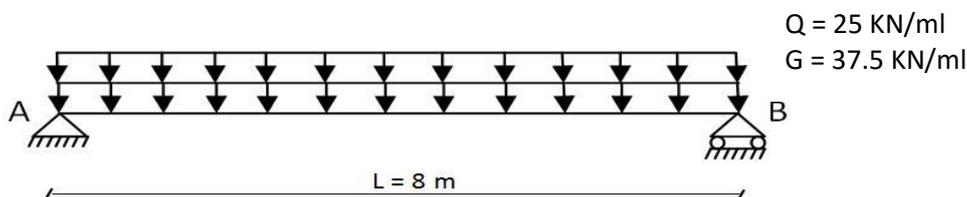
Figure 1. Statically determinate beam with simple supports.
