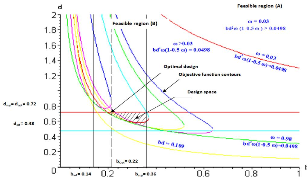
Fig. 3. Design space, reinforced concrete rectangular beam.
