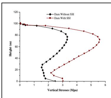
Fig. 10. Distribution of vertical stresses along dam height for model without SSI and model with SSI.
