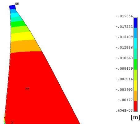
Fig.7. Maximum horizontal displacement contours of dam for model without SSI.
