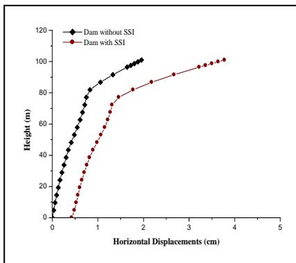
Fig. 5. Maximum horizontal displacements in upstream direction for model without SSI and model with SSI.
