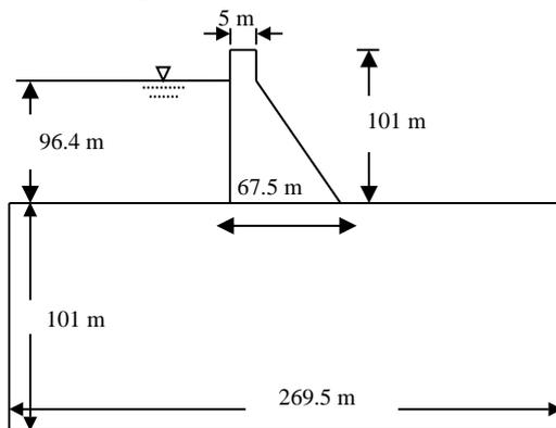
Fig. 1. Dam-foundation rock system.
