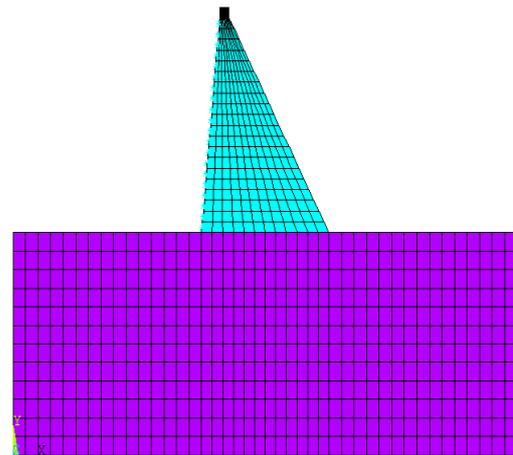
Fig. 3. Finite element model of dam-foundation rock system.
