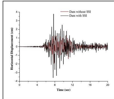
Fig. 6. Time history of horizontal displacement at crest of dam for model without SSI and model with SSI.
