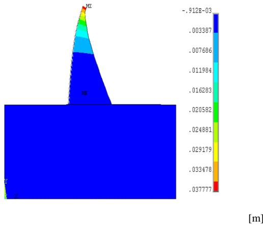
Fig.8. Maximum horizontal displacement contours of dam for model with SSI.
