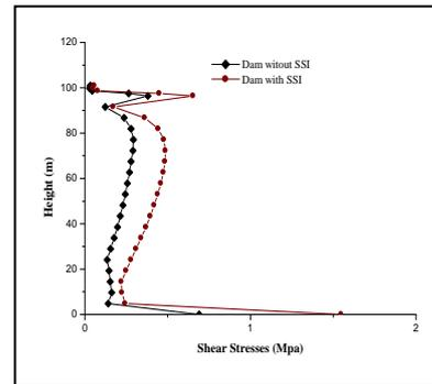
Fig. 11. Distribution of shear stresses along dam height for model without SSI and model with SSI.
