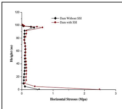
Fig. 9. Distribution of horizontal stresses along dam height for model without SSI and model with SSI.
