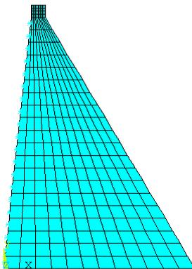
Fig. 2. Finite element model of dam alone.
