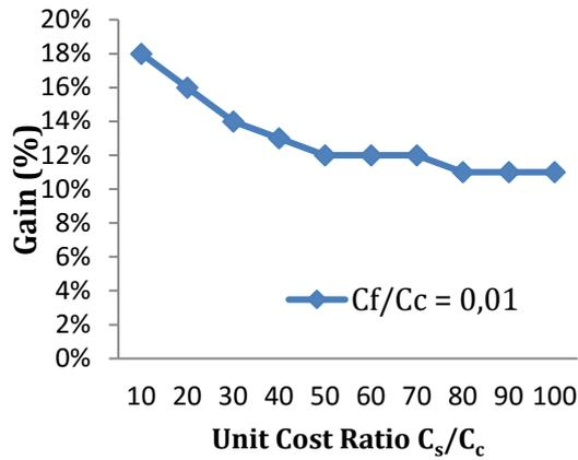
**Figure 4** Variation of relative gain in percentage (%) versus unit cost ratio  $C_s/C_c$  for a given cost ratio  $C_f/C_c=0.01$
