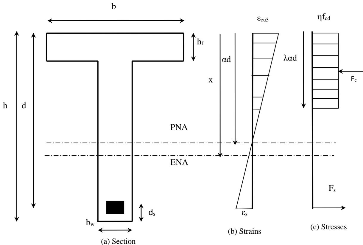
**Figure 1** (a) Typical T-beam cross section; (b) strains at ultimate limit state and (c) stresses at ultimate limit state.
