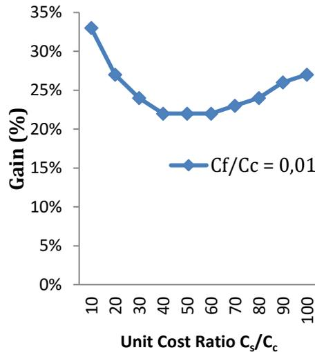
**Figure 2** Variation of relative gain in percentage (%) versus unit cost ratio  $C_s/C_c$  for a given cost ratio  $C_f/C_c = 0.01$
