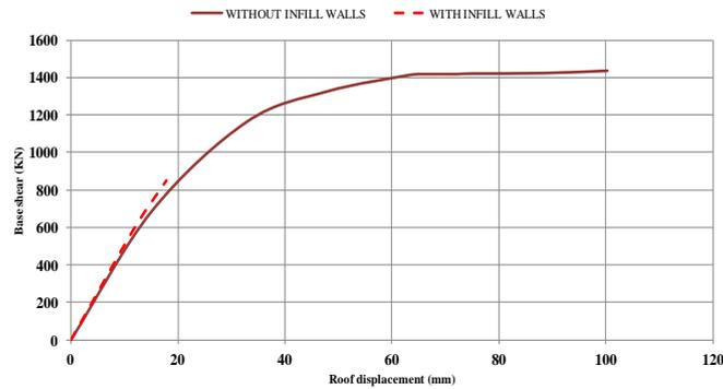
**Figure 5:** Capacity Curve for the transverse direction YY
