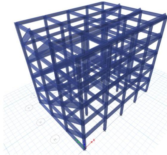
**Figure 4:** Three-dimensional model of the structure with infill walls
