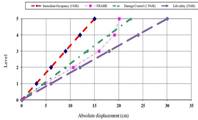
**Figure 6:** Absolute displacements for the transverse direction YY without infill walls
