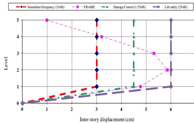
**Figure 8:** Interstory displacements for the transverse direction YY without infill walls
