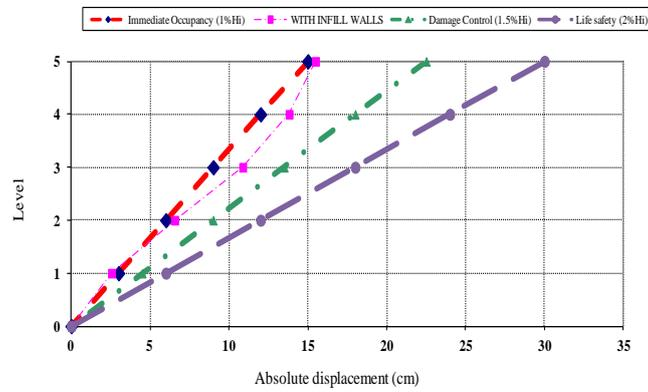
**Figure 7:** Absolute displacements for the transverse direction YY with infill walls
